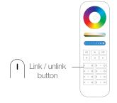
2. When the light is on, short press any zone of "  $\cap$ " 5 times (within 3 seconds), after connection.
